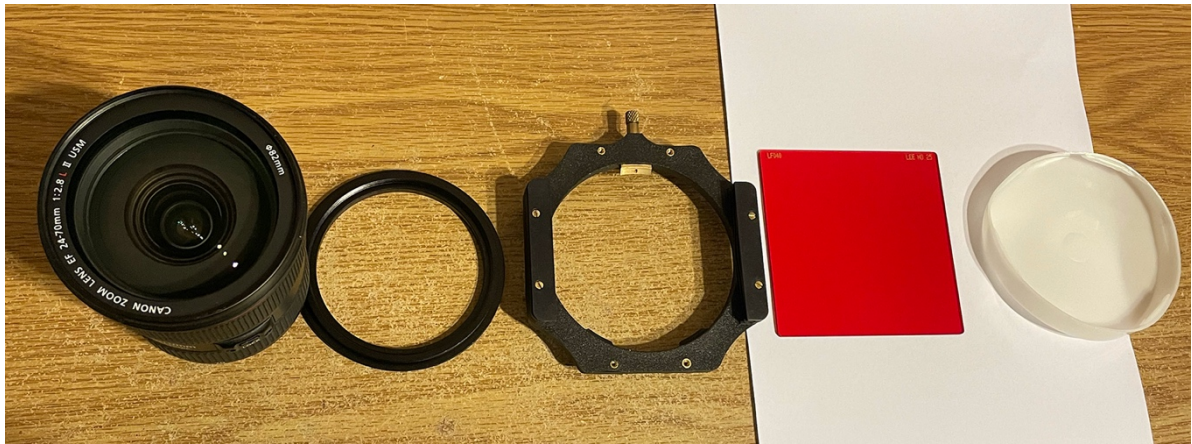
Here above is the Lee 100 system as an example. From left to right, lens, adapter ring to fit the thread size of the lens, holder, red filter and cap.
