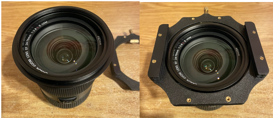
The adapter ring screws on the lens, the holder then attaches to the adapter ring.
